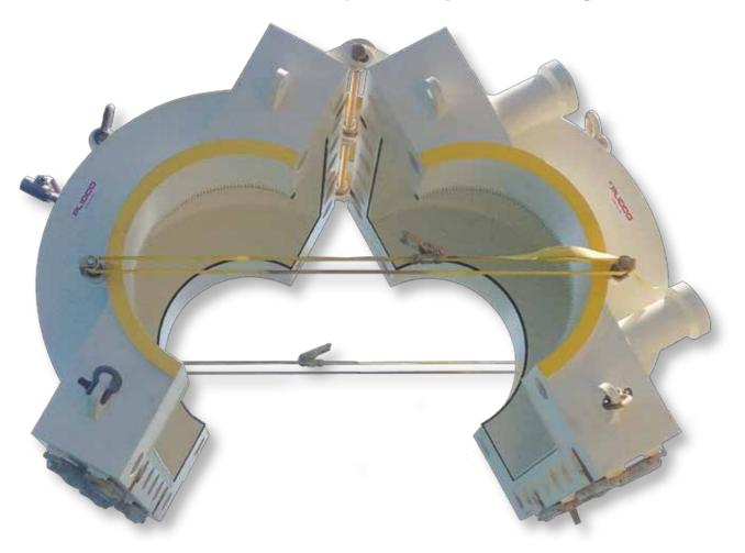
The PLIDCO<sup>®</sup> Flange Repair Split+Sleeve is used to fully encompass a flange set stopping the leak by sealing on the pipe beyond the flange welds. It has the ability to cover a wide variety of flange types and classes for both onshore and offshore applications. It is safe, easy to install, and as an option, can be welded while the line is in service.
