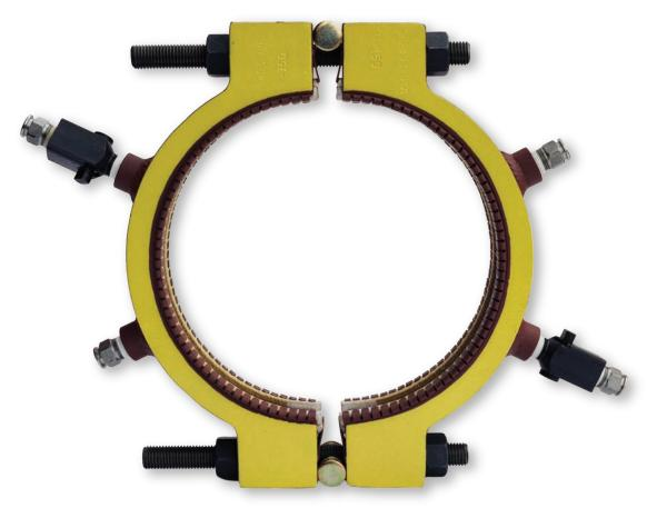
Plidco® Flange+Repair Rings can be installed by your own personnel. There is no drilling or altering of flanges. On a scheduled turnaround the Plidco® Flange+Repair Ring can be reconditioned and used again. Give us your conditions — pressure, temperature, fluid — and we will recommend the proper sealant and packing. Standard packing is non-asbestos aramid fiber.
